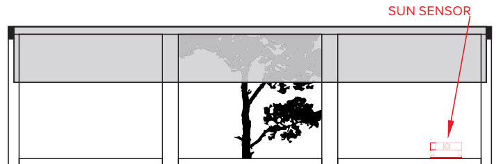
Correct - Sensor location clear of obstructing shadows
