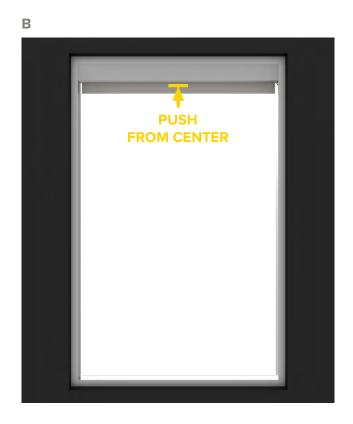
C If Bottom Rail raises at the desired speed, the correct number of preturns have been assigned.
